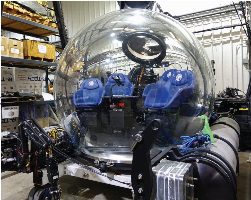
Below Left: World's deepest diving three-person acrylic hulled submersible capable of depths up to 1.4 miles
