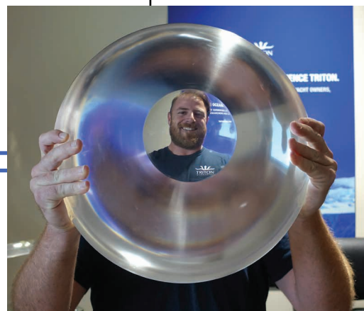
Below Right: Triton's Alex Aldrich looks through the acrylic porthole from the Triton Full Ocean Depth submersible capable of depths up to 6.8 miles
